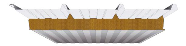
A notch in the eave area is recommended in order to rule out any possibility of the sheet metal shell lifting up from the insulation body (available at a surcharge). Similarly, a drip cap should be fitted in the eave area so as to prevent a capillary effect (only possible on the construction site).
