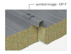
A notch in the eave area is required in order to rule out any possibility of the sheet metal shell lifting up from the insulation body (available at a surcharge). Similarly, a drip cap should be fitted in the eave area so as to prevent a capillary effect (only possible on the construction site).
