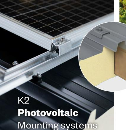
Fast and penetration-free installation, no fixation in the roof substructure required, controlled thermal longitudinal expansion without transferring tensile forces to the roof skin, system for simple and safe planning. DiBt PUR/PIR supporting approval number: Z-10.4-620 including PV mounting system to the BRUCHA panel roof PIR+ DP.
